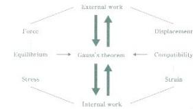
Virtual work and energy principles for trusses, beams and frames
